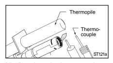
Pilot flame is weak - does not touch Thermocouple.
